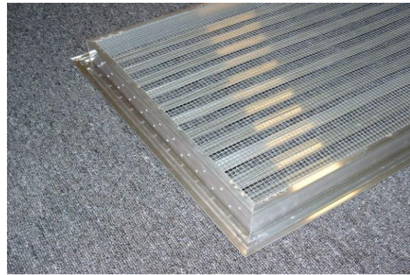
Louver is 2.0" in depth with a 1-1/4" front mounting flange
